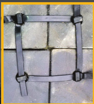
Correct way to use cable ties
