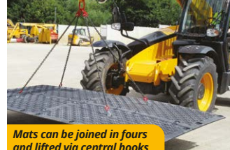
Mats can be joined in fours and lifted via central hooks
