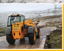
Subject to firm, dry ground conditions, SignaRoad<sup>®</sup> mats are usually comfortable with vehicles up to 60 tonnes UDL (Uniformly Distributed Load). Heavier vehicles up to 100 tonnes may be used with caution for short term access in dry weather. However, it is the user's responsibility to assess the load-bearing capacity of the ground, and to only operate vehicles within the weight that the ground is capable of safely supporting.
